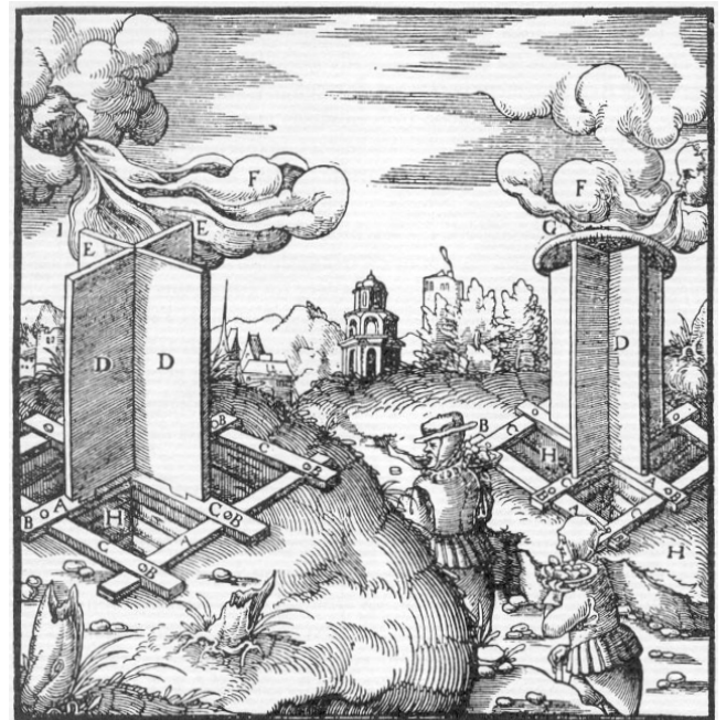
Figure 8: Other forms of wind deflectors; note that these do not allow extraction (after Agricola; France-Lanord 1992, 164).
