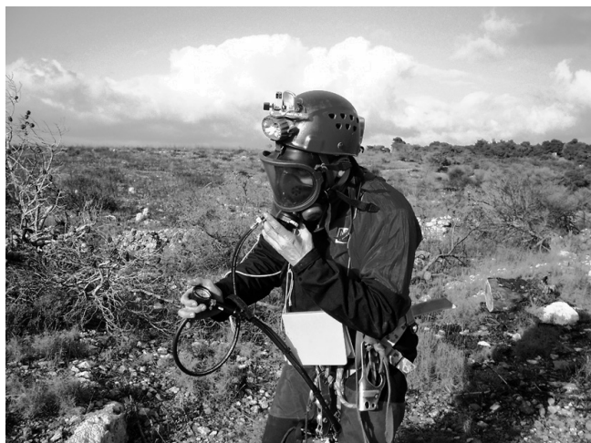
Figure 3: The self-contained breathing apparatus (SCBA) used when exploring the Laurion mines (Fenzy ARI).
