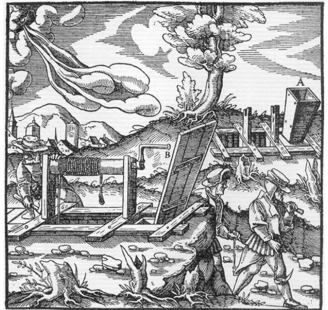
Figure 7: Wind deflector and chimney (after Agricola; France-Lanord 1992, 165).
