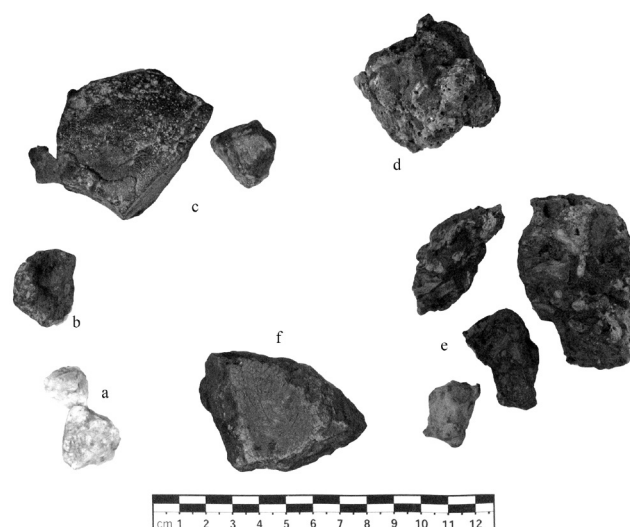
Figure 5: A (substantial) sample of the materials recovered in the workshop topsoil: a. quartz, b. haematite, c. slag fragment, d. vitrified ceramic fragment, e. furnace wall fragment, f. tuyère fragment (curved interior uppermost).
