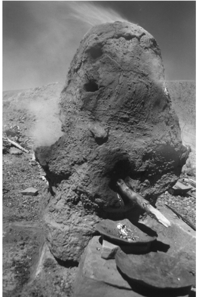
Figure 6: The huayrachina in action. Lead is flowing from the top hole at the bottom of the shaft onto a shallow iron dish (bottom right).
