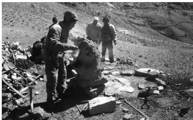
Figure 7: Carlos Cuiza attends to his smelt, topping up charge and when necessary feeding slag back into the huayrachina .
