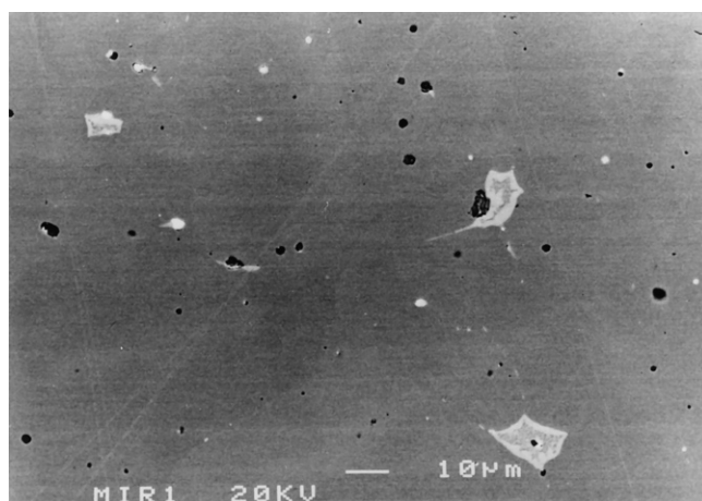
Figure 4: Backscattered SEM image showing sulphide inclusions (black), ( \alpha+\delta ) eutectoid second phase (pale grey) and small round lead-rich inclusions (white). Scale bar: 10µm.
