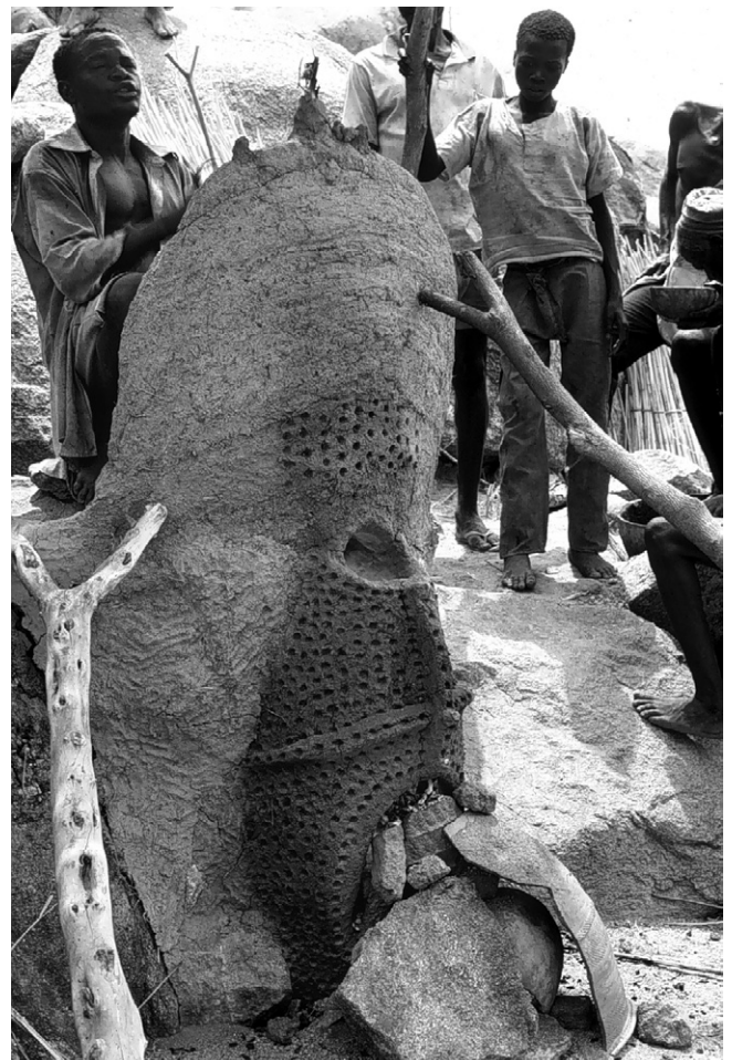
Figure 4: Plata furnace during a re-enactment arranged for the MAP team by Scott MacEachern in 1989 (David 1995). The shaft opening is poorly blocked, resulting in considerable heat loss. Photo David Killick.
