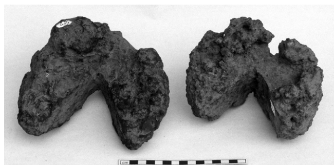
Figure 19: Two axe-cut blooms from the Samanalawewa project area. Scale bar 150mm.
