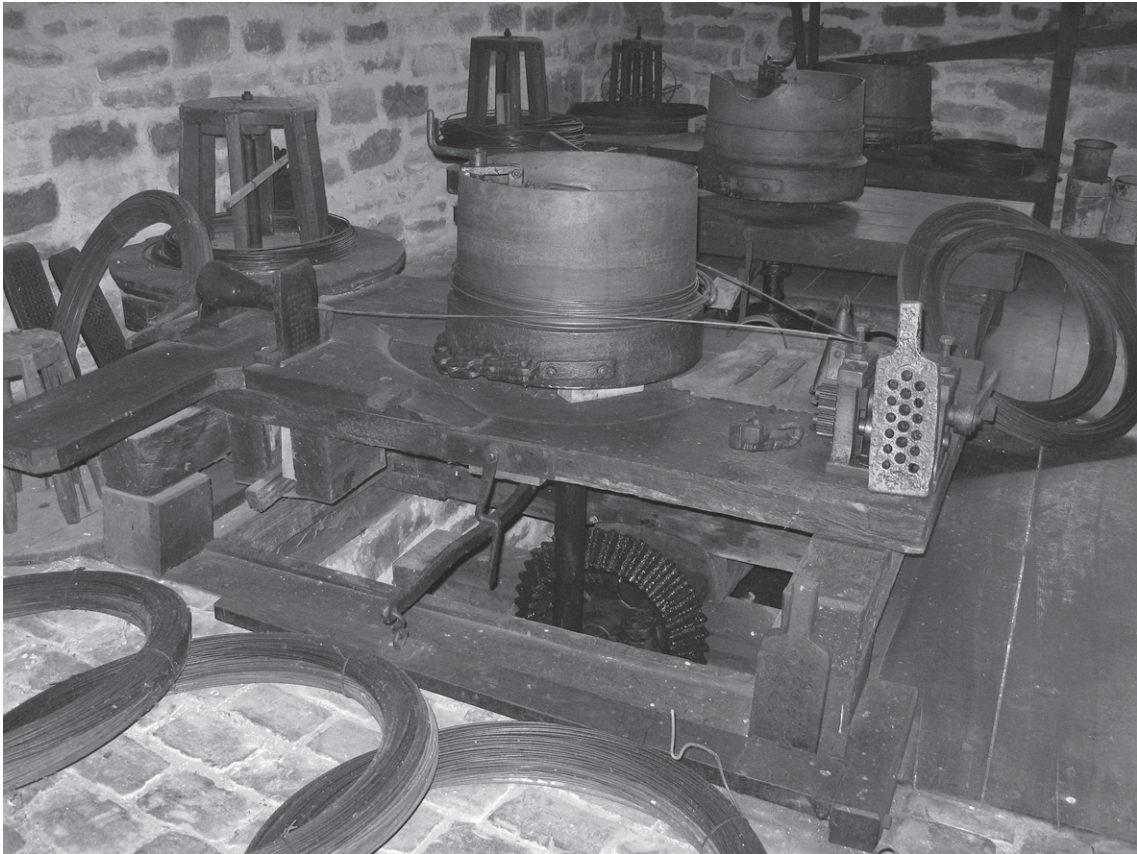
Figure 6: Interior of a reconstructed German wire mill at Hagen, Westphalia, showing wire being taken from a swift (to the left) through a draw plate and then taken up on a drum driven by the bevel gearing of the water-powered drive. A spare draw plate can be seen propped up at the right-hand front corner of the bench. Two further sets of wire-drawing equipment are visible in the background.
