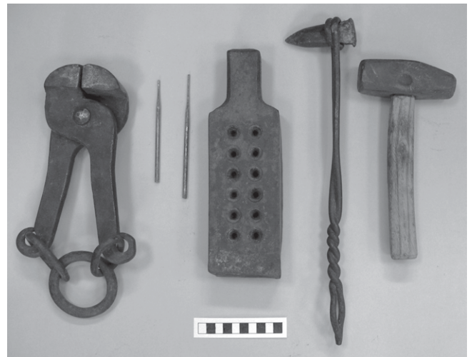
Figure 10: Left to right: dog for gripping wire during the first stage of drawing; two wire-drawer's punches; wortle plate; wortle plate pricker's punch; battering hammer. Scale 100mm. (Hawley Tool Collection).
