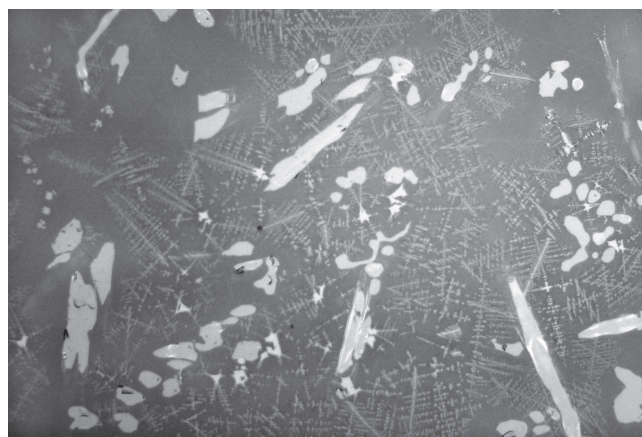
Figure 10: Polished section of slagged tuyère tip SK2 from Smelters Kop, showing light cassiterite crystals in glass, with fine fayalite dendrites (image width 0.3mm).
