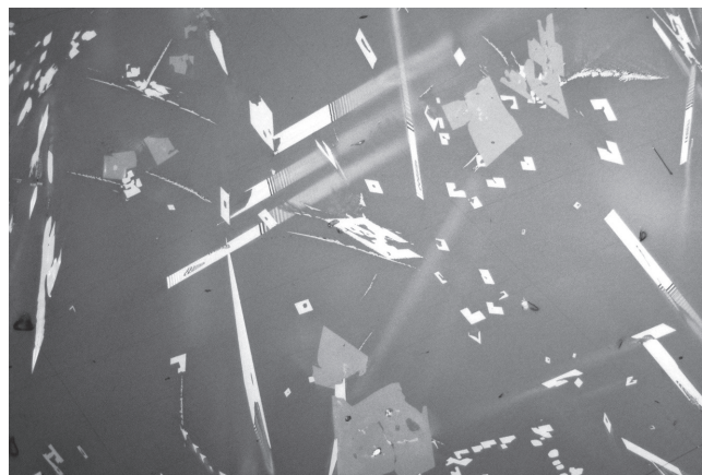
Figure 12: Polished section of tin smelting slag nodule SK4 from Smelters Kop, showing blocky zircon crystals (medium grey) and laths of rutile (light grey) in glass (image width 0.3mm).
