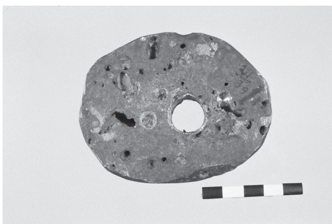
Figure 4: Tin bun ingot (Wits 21/39/1) from Rooiberg. The central hole and the one to the right of it were drilled by earlier analysts. The other holes are gas porosity (scale bar 50mm).
