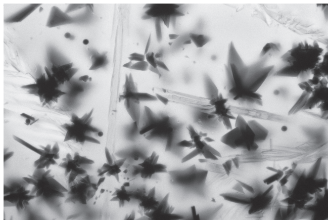
Figure 11: Thin section of tin smelting slag nodule SK3 from Smelters Kop. The light laths are fayalite in a pale glass, with stellate rosettes consisting of blades of titaniferous augite around opaque cores of spinel (image width 0.4mm).
