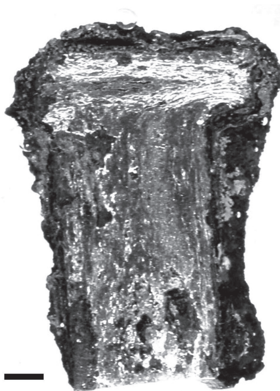
Figure 12: The asymmetrical shear structure found in the head of nail 34, recovered at the Woodhouse site, Greene Farm excavation, Warwick, Rhode Island, is interpreted as resulting from imperfect alignment of the heading die in the one-operation machine that made this nail. Nital etch; length of scale bar 2mm.
