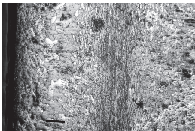
Figure 11: At higher magnification the elongation of the ferrite grains in the shear band shown in Fig 10 is revealed. Iron between the shear band and the top of the head is undeformed, as is the iron below, except for the outward bend toward the edges of the nail. Nital etch; length of scale bar 0.2mm.
