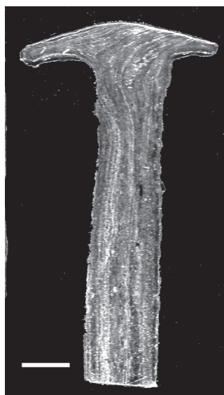
Figure 5: Hand-forged nail 22, from the early-19th-century Glebe House, Woodbury, Connecticut. The folded structure in the head resulted from the initial diagonal blow struck by the smith with the nail in the header. Nital etch; length of scale bar 2mm.
