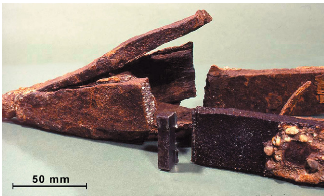
Figure 1: The broken pile-shoe with a sawn-off slice containing the upper fracture surface of the recent break.
