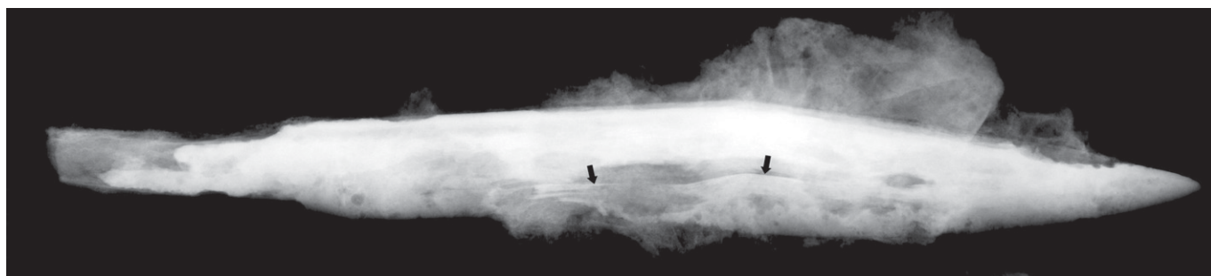
Figure 4: X-radiograph of knife 434 from St Mary's Stadium, Southampton. Note the 'spotted' texture indicative of steel in the cutting edge (bottom strip) and a distinct weld line (arrowed) running along the blade. Length 166mm.
