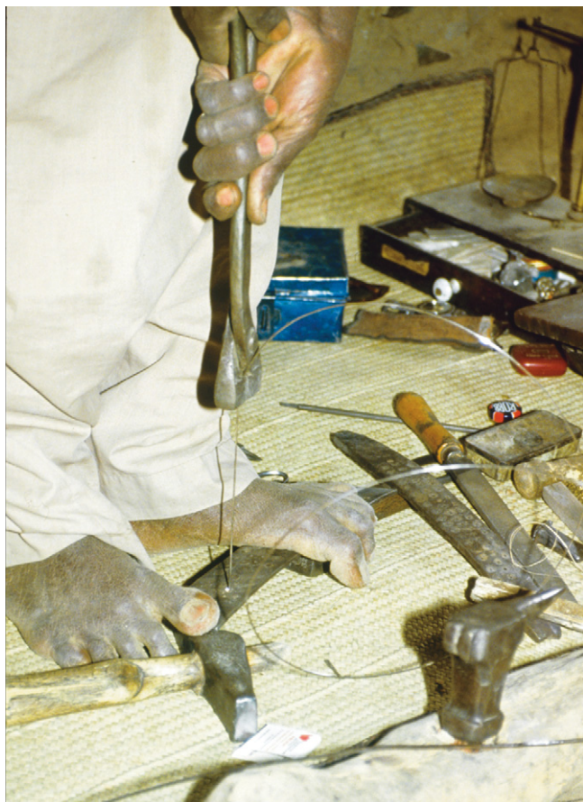
Figure 10: Wire drawing in Mali; the draw plate is held between the feet.
