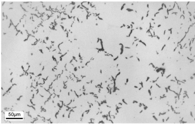
Figure 5: Unetched polished section on the right arm of Dawson's statuette with fine graphite flakes distributed interdendritically.
