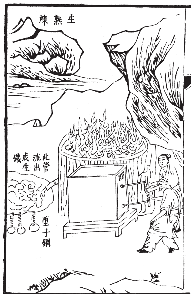
Figure 8: Illustration of a blast furnace in the 17th-century technological compendium Tian-gong kai-wu , by Song Yingxing.
