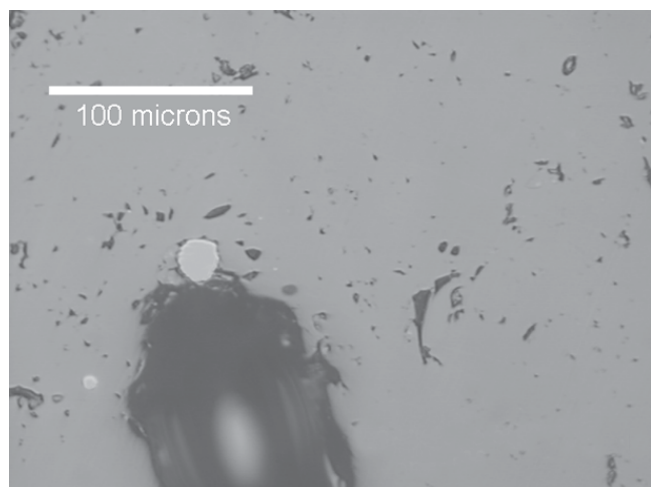
Figure 7: Vitreous slag from Longstone (sample 24) showing tin prills. Magnification \times 270 .
