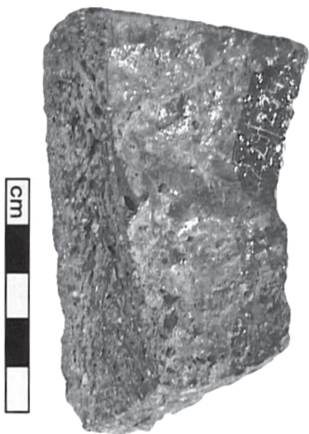
Figure 10: Inner surface of a type C crucible. Note the line of a thick layer of slag parallel to the rim, probably floating on the molten brass. Scale bar 50mm.
