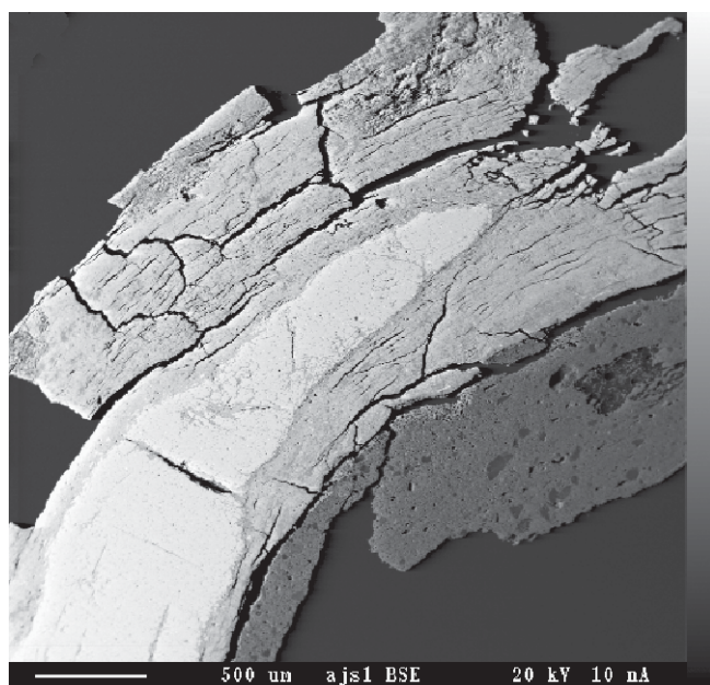
Figure 1: Low magnification backscattered SEM image of the cross section of the bead, showing fresh unweathered metallic antimony areas (light grey), the oxidized outer surface (mid grey) and remnant ceramic core (speckled dark grey).
