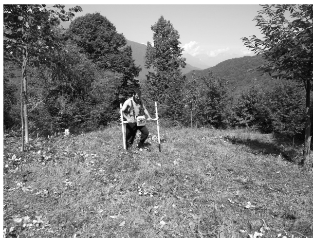
Figure 11: Looking south across the working area of the copper smelting site Dogurashi III with geophysics underway. The survey suggests that a possible smelting furnace lies beneath the apex of the low mound with slaggy waste tipped to the west (right) down the mountainside.
