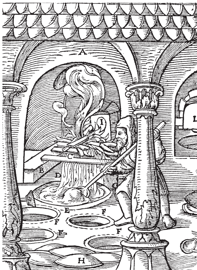
Figure 2: Carniolan process of lead smelting as illustrated by Agricola in De Re Metallica .
