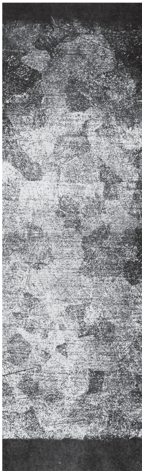
Figure 5: Sample C (pseudo-medieval steel) after quenching and tempering for one hour at 500°C (x70)
