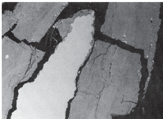
Fig 2: Sword sample, showing sound metal core and fragmented corroded surfaces (x 5).
