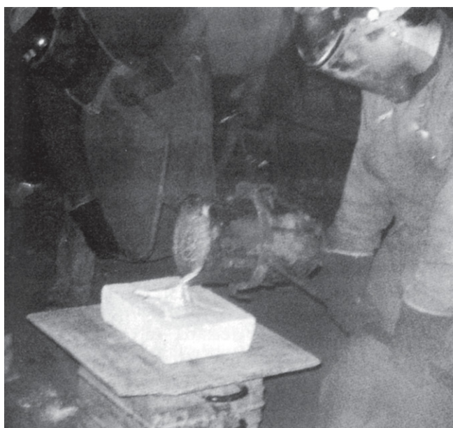
Fig 5: Pouring molten copper into the replica mould.
