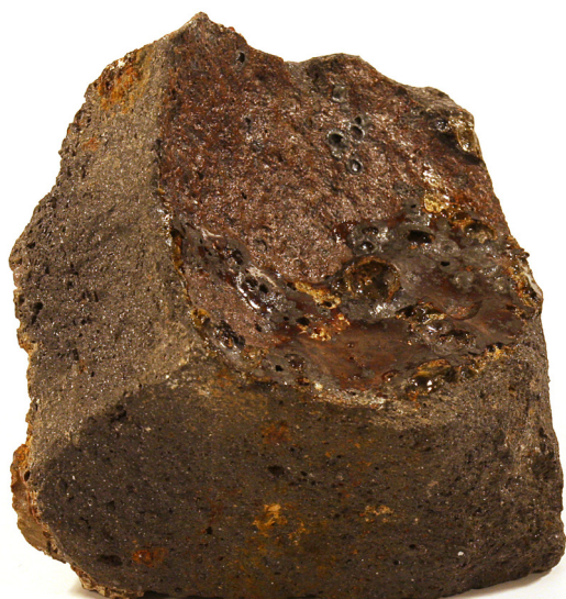
Figure 1: Fragment of crucible 5377-1. Note the internal coating of manganese silicate slag.
