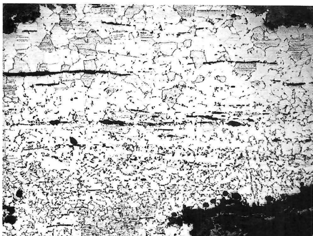
Fig 12: Section near thinner end of Fig 11. Mag. X80. The upper part shows coarse ferrite grains (ASTM 2-3), low in carbon, which were near the outer surface visible in Fig 1. The lower part shows fine ferrite grains (ASTM 7) and higher carbon content. These formed a central layer through the thickness of the spearhead. Black, elongated particles are slag.
