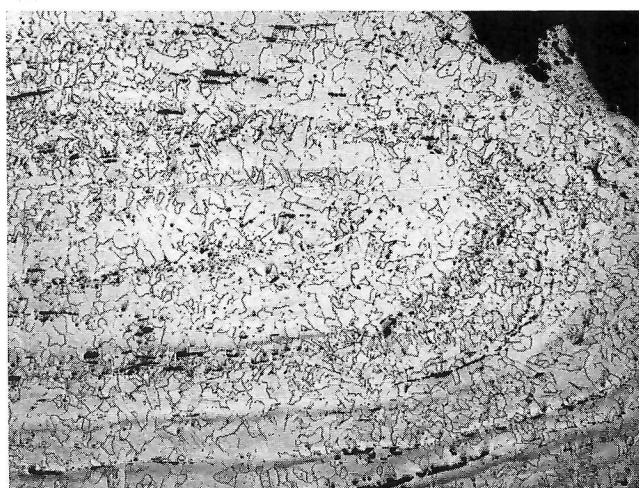
Fig 9: Enlarged area from Fig 8. Mag. X40. Shows uniform ferrite grain size. Elongated black particles are slag. Semi-circular pattern of laminations indicates folding to form the blade and the line of small dark inclusions centre left represents oxide inclusions along the weld line.
