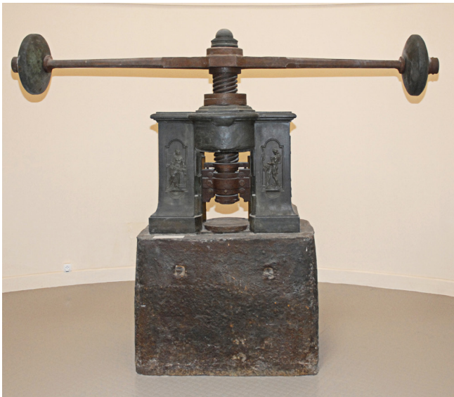
Figure 4: Screw press, known as le balancier Delaunay ; bronze, steel, lead, 1697. © Musée de la Monnaie, Paris.
