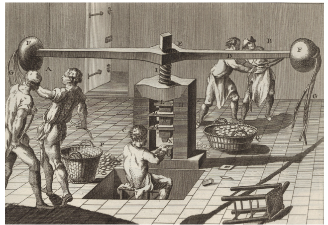
Figure 17: A screw press (Diderot and d'Alembert 2017, 'Monnoyage' plate XV, detail). By courtesy of the ARTFL Encyclopédie Project, University of Chicago.
