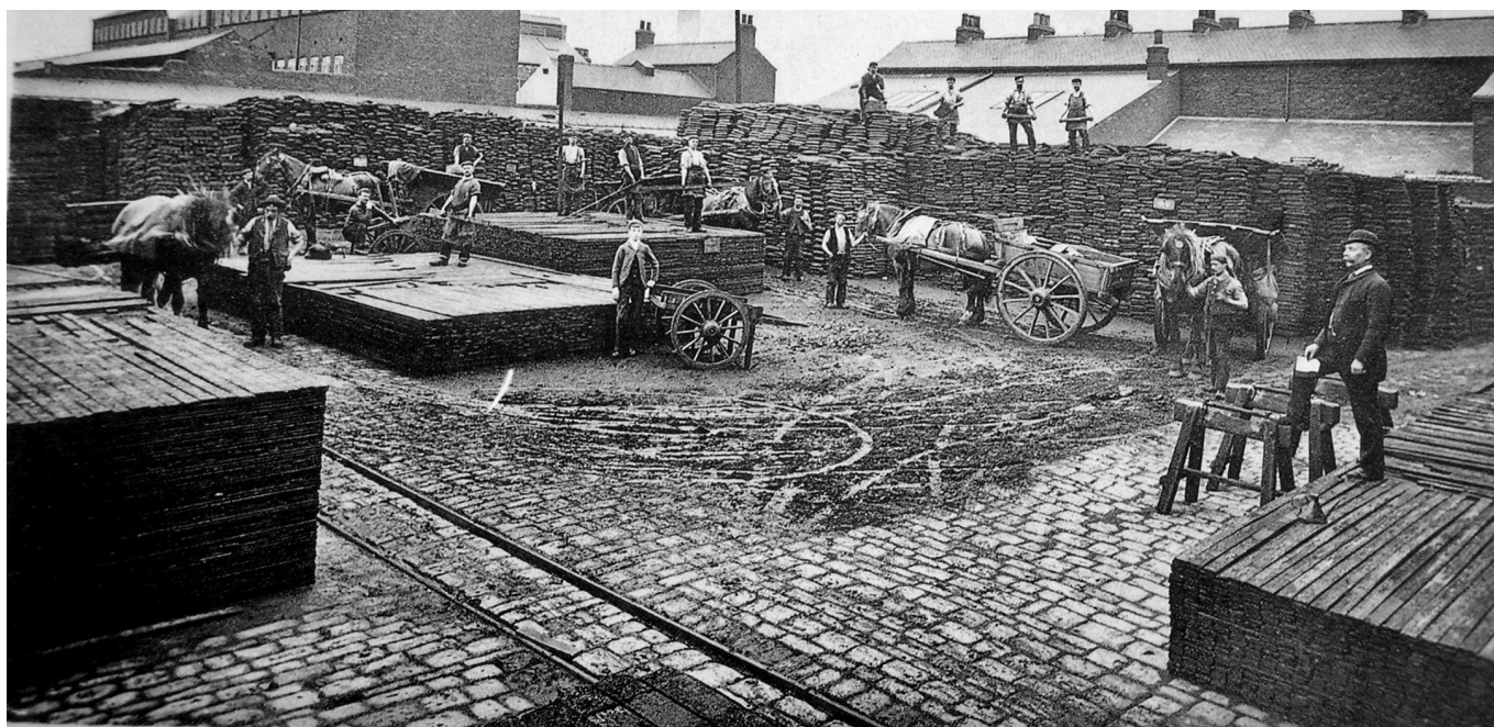
Figure 4: Swedish wrought iron for conversion to crucible steel c1900. Photograph courtesy of Ken Hawley Tool Collection Trust.
