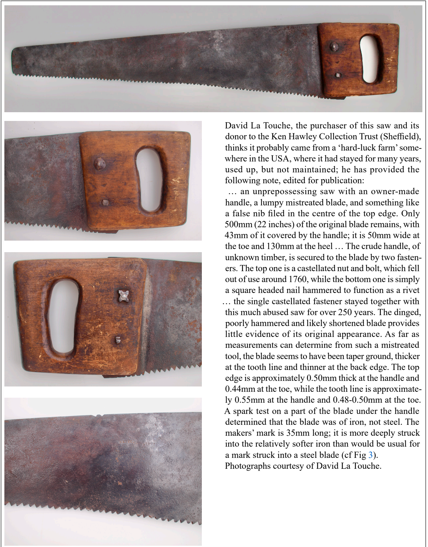
Figure 2: Iron hand saw by Kenyons & Jones c1757.
