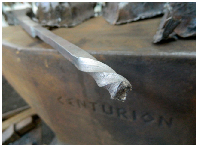
Figure 10: Low-phosphorus ductile fracture.
