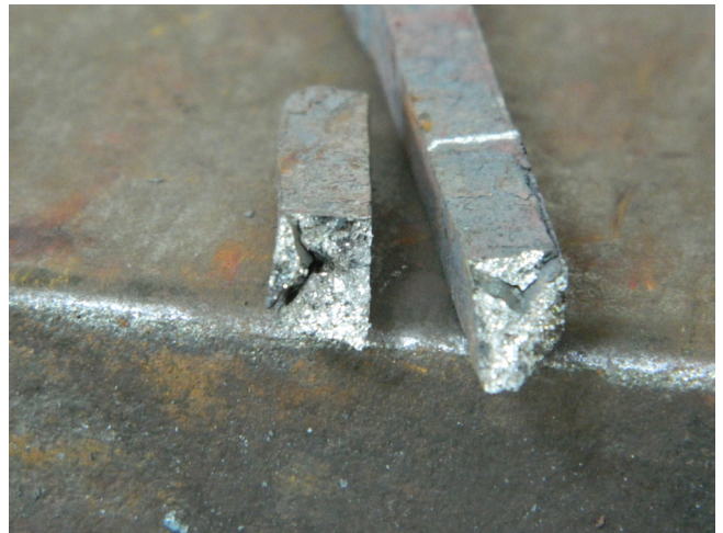
Figure 9: High-phosphorus brittle fracture. You can also see here the typical diagonal cracks from the corners discussed in part three.
