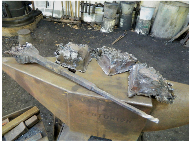
Figure 8: Bar forged direct from bloom.
