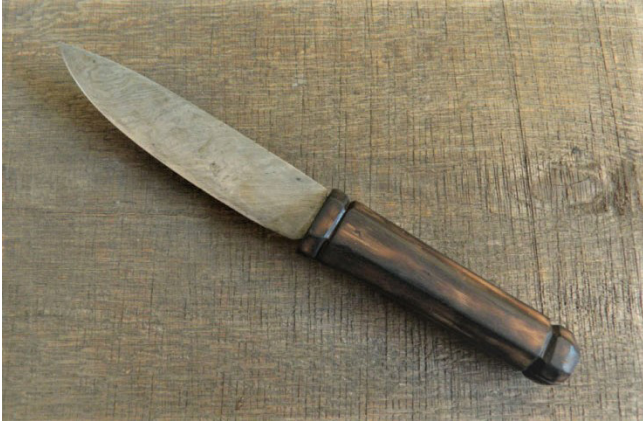
Figure 6: This knife was forged from low-carbon, medium-phosphorus iron, and the edge was cold hammered before sharpening. I have used it to gut, skin, and butcher several deer.
