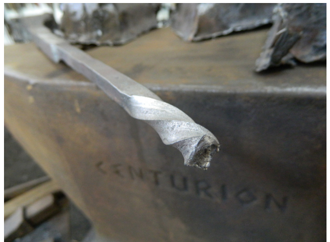
Figure 10: Low-phosphorus ductile fracture.
