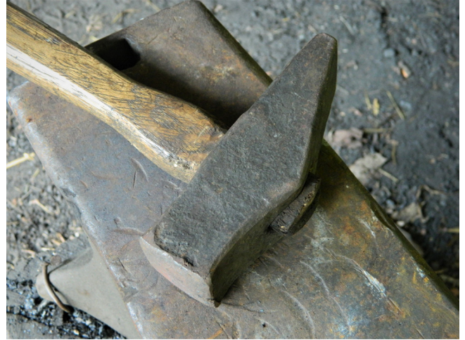
Figure 7: Hammer of low-carbon phosphoric iron, showing only mild mushrooming after many years of use (hot forging only).
