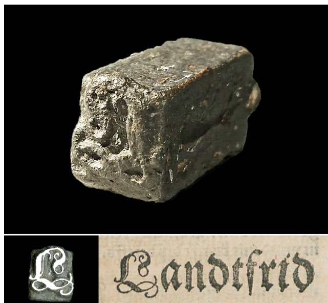
Figure 3: Type piece with a sprue (just visible at the back) found in a latrine of the late 16th century at Hintere Flachsmarktstraße in Mainz (point size 13.6mm, type height 25.5mm, set width 11.3mm). Below, the reflected face of the type is compared with an upper-case L in a printing by Franz Behem from 1566/1573.
