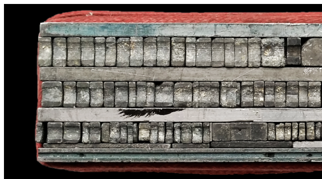
Figure 16: The underside of the type from Oberursel (cf Fig 6) showing their feet and grooves. Parallel scratches running from one type piece to the next indicate simultaneous working with a plane within a single workshop. The type pieces hence belong to the same set. Image width c50mm.
