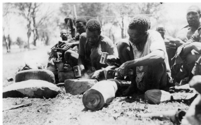
Figure 6: Njanja smithing operations, here using modern hammers (?), at the same event as shown in Figure 5. Note the bellows-blown forge to the left. (Photo: National Museums and Monuments of Zimbabwe).
