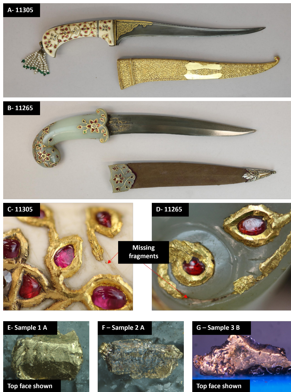
Figure 1: A shows the T-shaped dagger (RCIN 11305). B is the nephrite hilted dagger (RCIN 11265). C is a macro image of kundan settings from the dagger RCIN 11305. D is a macro image of kundan settings of RCIN 11265 with missing fragments and residual lac in the setting. E is a fragment from RCIN 11305: the top cut face is shown. F shows a fragment from the same dagger with surface discolouration from creeping sulphide corrosion. G shows the top face of a sample from the dagger RCIN 11265. (A-B reproduced with permission from Royal Collection Trust / © His Majesty King Charles III, 2023).
