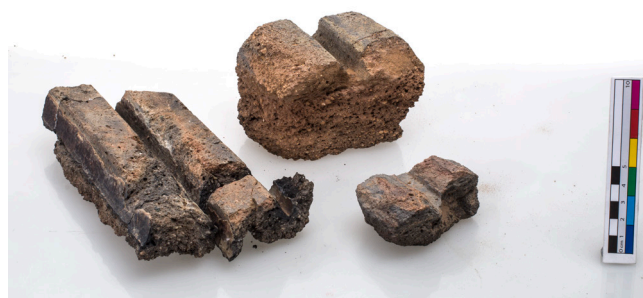
Figure 20: Fragments of ingot moulds recorded at Tamdult used to produce long brass ingots. The one on the left has a V-shaped cross-section, the one at the top a trapezoid section.
