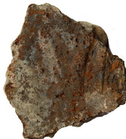
GST-cai-8: The inner surface is dark red, with clear honeycombing marks. On the inner surface is a fragment of the character 太 with the same form and size as the corresponding character on the bridge pier. Dimensions 263×245mm, thickness 40–60mm.
