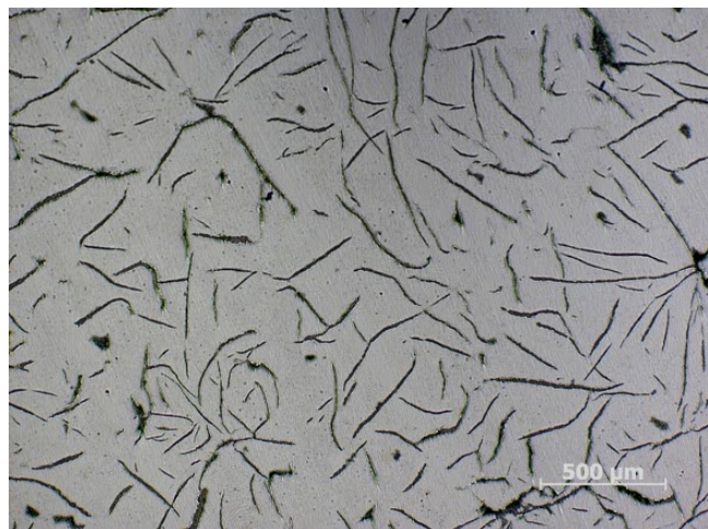
Figure 6: Flake graphite (dark) in metallic matrix. Unetched. Scale bar 500μm.
