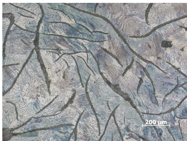
Figure 7: Flake graphite (dark) in pearlite matrix. Etched with nital. Scale bar 200μm.
