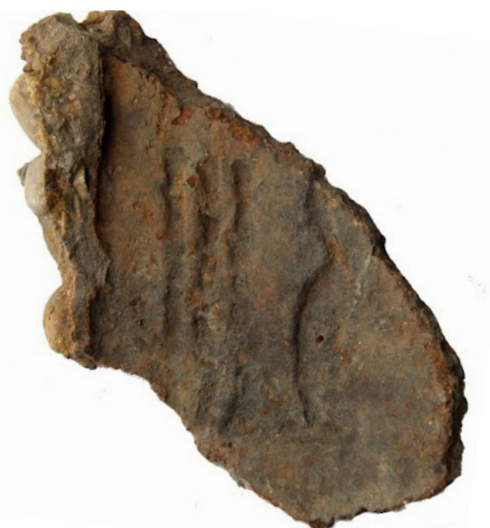
GST-cai-6: On the inner surface is a fragment of the character 江 with the same form and size as the corresponding character on the bridge pier. To the left of the character is an approximately rectangular protuberance, 60×40mm, 20mm thick. Judging from the position of the fragment in the mould, the protuberance joins with the core for the recess at the upper part of the casting. Dimensions 260×180mm, thickness 40–70mm.
