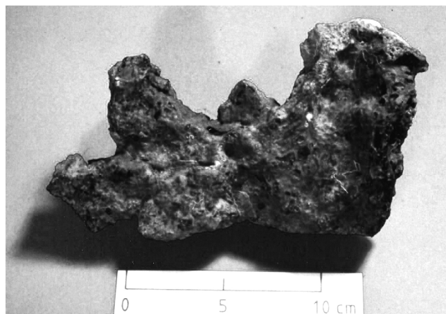
Figure 8: Half of a fired clay air inlet, found at the Vårhussetra site.
