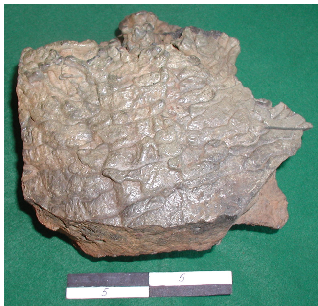
Figure 6: Piece of slag from the cold, stone-lined slag pit. Note the ripples. Each ripple may represent c10kg of slag. Scale bar 100mm.
