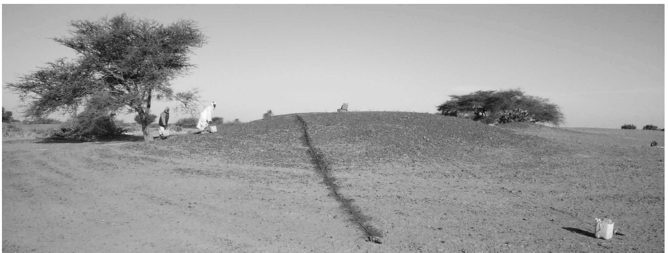
Figure 3: View from west towards the slag heap H800 during the resistivity measurements. The electrodes had to be watered to reduce the ground-coupling problems. The circular lining around the heap indicates different water levels of the annual flooding of the Nile.
