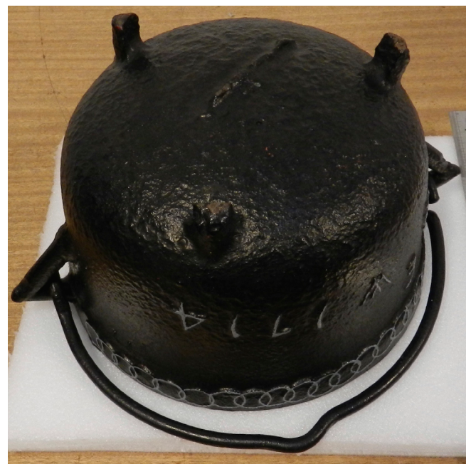
Figure 14: The underside of the pot in Figure 13 showing the lack of both a vertical parting line and one across the bottom; it could not have been made with loam and thus not with charcoal-iron.
