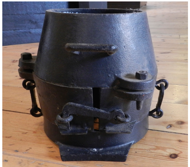
Figure 11: Set of iron moulding boxes for the manufacture of pots like those shown in Figures 9 and 10. IGMT Acc Num 1997.623–5, 300mm diameter.
