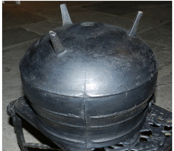
Figure 12: A spurious, much fainter line across the base of a green sand moulded pot, revealing that the original pattern was made with loam. John Edwards collection. 300mm diameter.
