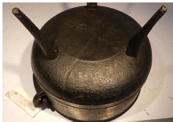
Figure 4: An 18th-century loam moulded pot, showing the characteristic parting line. MM Acc Num 38128. 200mm diameter.
