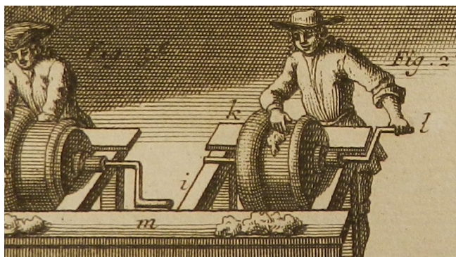
Figure 2: The first stage in making a loam mould: forming the core with a lathe and a shaped board. From Duhamel de Monceau 1774.
