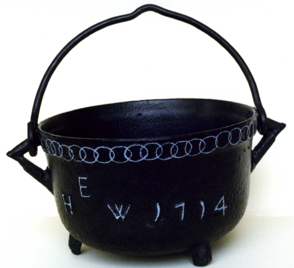
Figure 13: The oldest known coke-iron casting. It is a genuine Darby casting, made just six years after he first used coke in his furnace. IGMT Acc Num CBD59.74. 265mm diameter.
