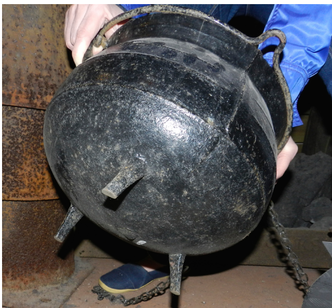
Figure 10: The pot shown in Figure 9; note the absence of any loam-type line across its base.
