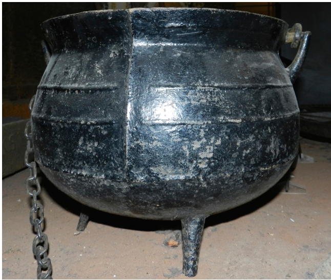
Figure 9: Cast iron pot made using a mould of the type shown in Figure 8. The two upper horizontal lines are decoration but the bottom one is a parting line, as is the vertical line. IGMT Acc Num 1993.5731, 400mm diameter.
