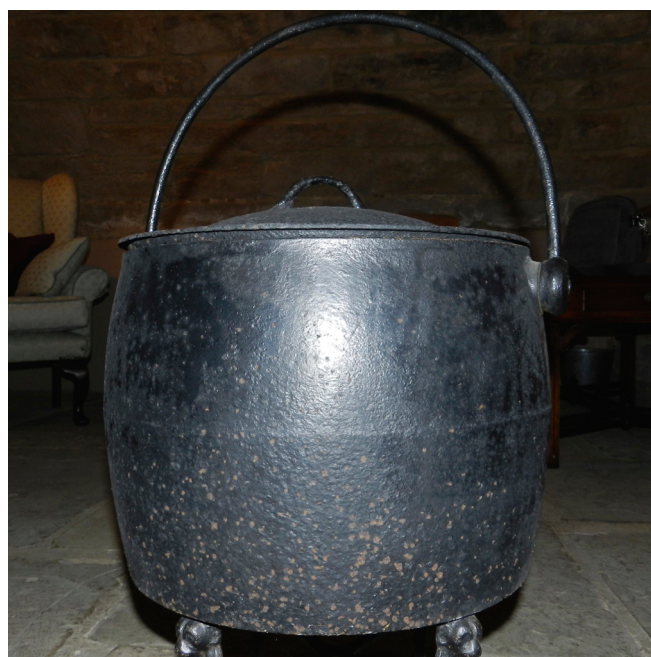
Figure 7: Pot made from a three part mould, with a central horizontal parting line. John Edwards collection. 320mm diameter
